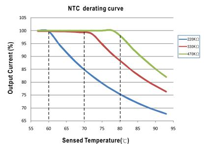
© LCM-60 can still be operated normally when the NTC resistor is not connected and the value of output current will be the current level selected through the DIP switch.
