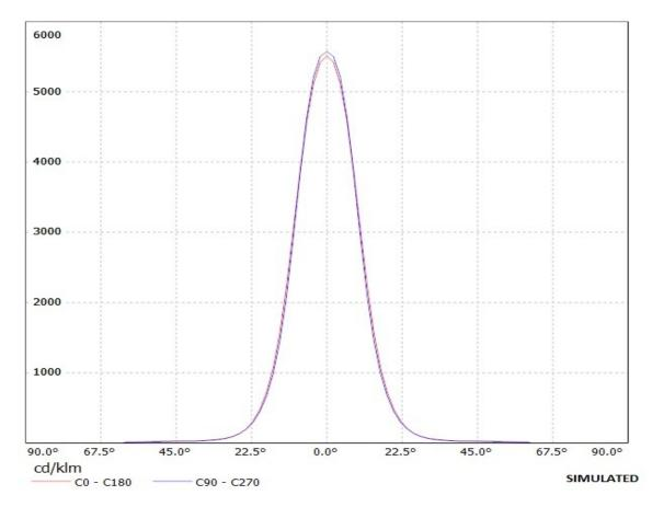
Luminaire: Ledil Oy FA10613\_LM1-RS FA10613\_LM1-RS Lamps: 1 x Cree MC-E (White)
