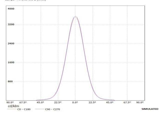
Luminaire: Ledil Oy FA10615\_LM1-REC FA10615\_LM1-REC Lamps: 1 x Cree MC-E (white)
