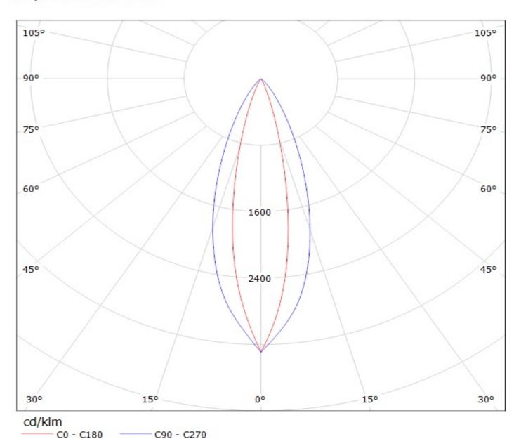
Luminaire: Ledil Oy FA10650\_LM1-D FA10650\_LM1-D Lamps: 1 x Cree MC-E
