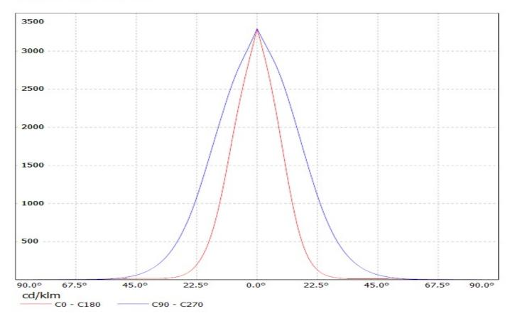
Luminaire: Ledil Oy FA10650\_LM1-D FA10650\_LM1-D Lamps: 1 x Cree MC-E
